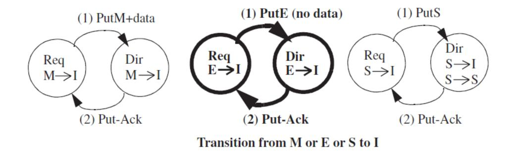
Fig 8.6 from D. Sorin et al. A Primer on Memory Consistency and Cache Coherence.
