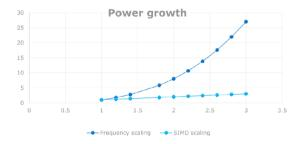
Wider SIMD -- Linear increase in area and power Wider superscalar – Quadratic increase in area and power Higher frequency – Cubic increase in power
