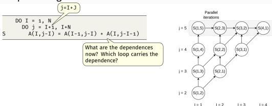
Loop skewing skews the inner loop relative to the outer loop by adding the index of the outer loop times a skewing factor f to the bounds of the inner loop and subtracting the same value from all the uses of the inner loop index
