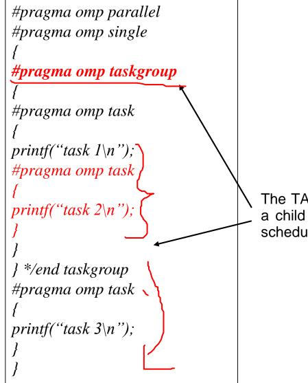
The TASKGROUP construct ensures task 2, which is a child of task 1, is also completed before task 3 is scheduled.
