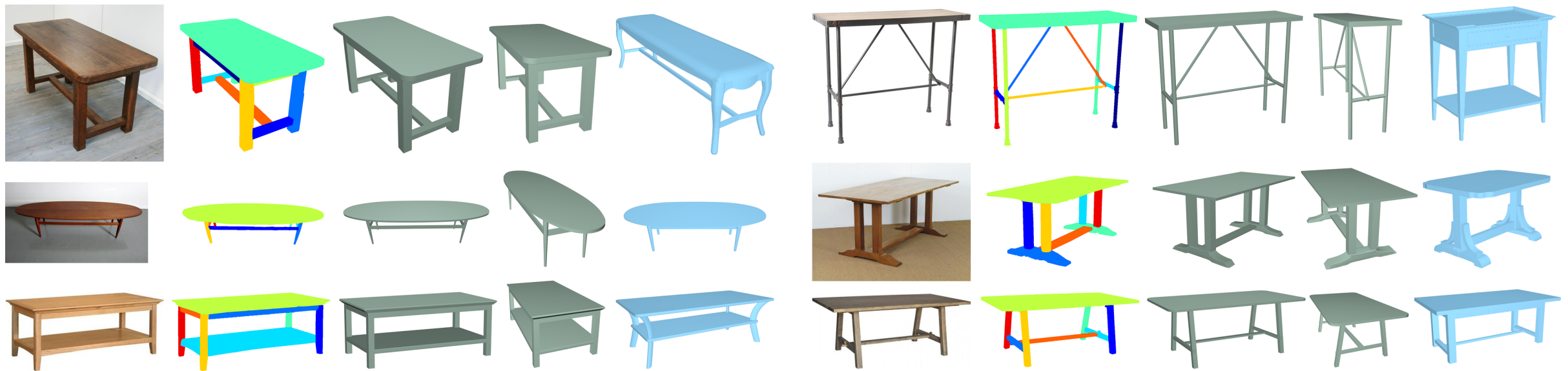
Figure 8: Results on four datasets. From left to right in each column: Web image, computed segmentation, 3D model reconstructed by our approach (two views, green), and closest pre-existing model, shown for reference (blue).
