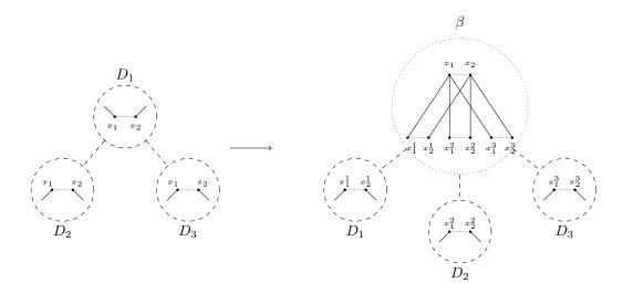
**Figure 1** (Left)A separating set  $\{x_1, x_2\}$  is shared by components  $D_1, D_2$  and  $D_3$ . (Right) Replace them by adding the gadget  $\beta$  and connect  $D_1, D_2$  and  $D_3$  to  $\beta$ .
