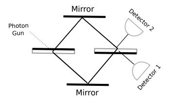
Fig. 2. Mach-Zehnder interferometer: Black edge is the reflecting edge in both beam splitter as well as the mirror. Notice that the "up" beam has to go through one more reflection.
