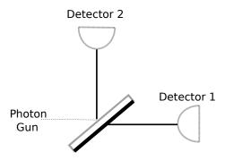
Fig. 3. A beam splitter and two detectors
