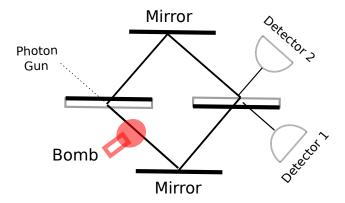
Fig. 4. Elitzur Vaidman bomb tester: how to test a bomb without exploding it.
