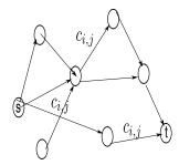
Fig. 1. Max flow problem: Capacities, source and sink.
