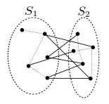
Fig. 1. Example of a cut with edges in the cut shown with solid line
