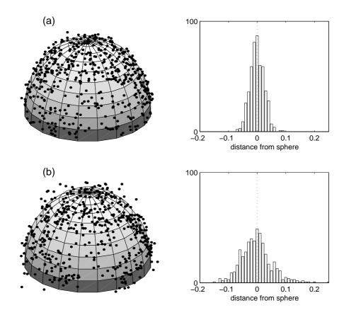
**Figure 2:** Modelling noisy data on a hemisphere. (a) On the left, the synthetic data, on the right, a histogram of the Euclidean distances of each data point to the sphere. (b) Similarly for data generated from the fitted PPCA mixture model.
