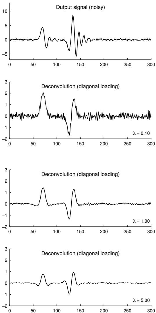
Figure 5: Deconvolution of noisy data by diagonal loading.
