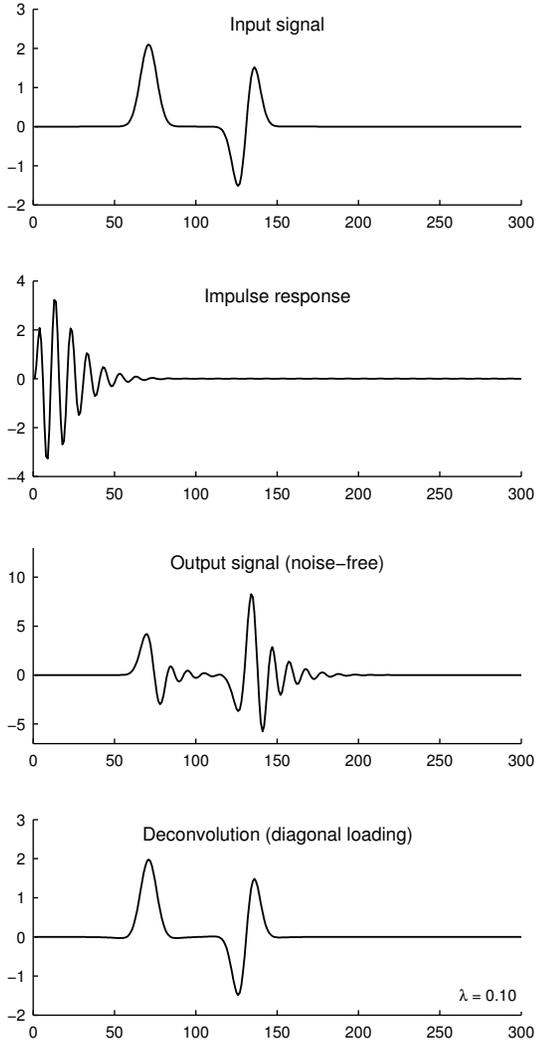
Figure 4: Deconvolution of noise-free data by diagonal loading.
