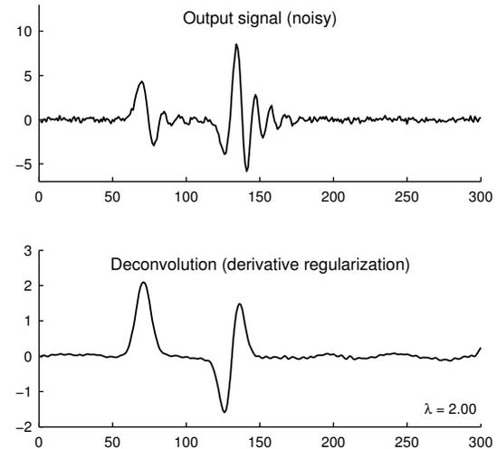
Figure 6: Deconvolution of noisy data by derivative regularization.
