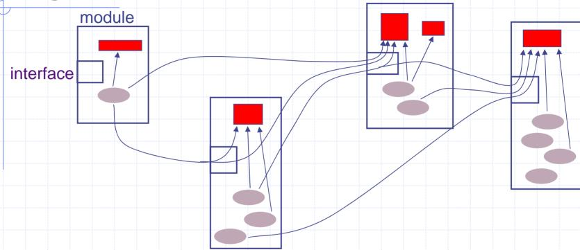
Each module embodies its own resources and is mapped on to its own hardware – no time-multiplexing
