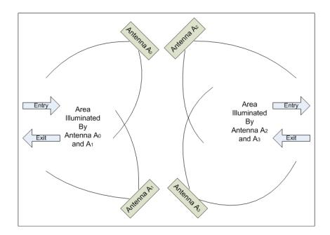
Figure 4.2: Antenna Placement and Orientation at the Room Entrance
