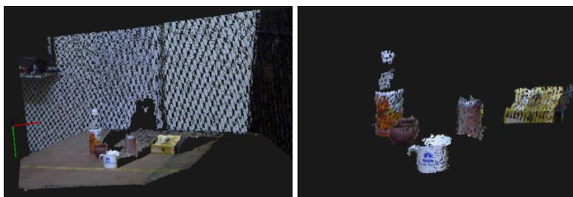
**Figure A.2:** The input pointcloud, and result after filtering the background and the tabletop
