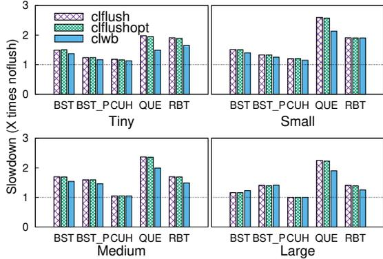
Fig. 5: Performance slowdown with different data consistency methods in x86-64 systems. Y-axis values are slowdown normalized to noflush (lower the better)
