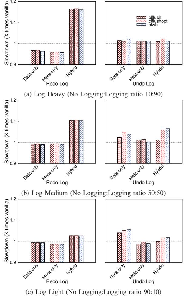
Fig. 7: Influence of data consistency methods based on nature of update operations for different logging requirements in x86-64. Y-axis values are speedup w.r.t. vanilla case of no logging (lower the better).
