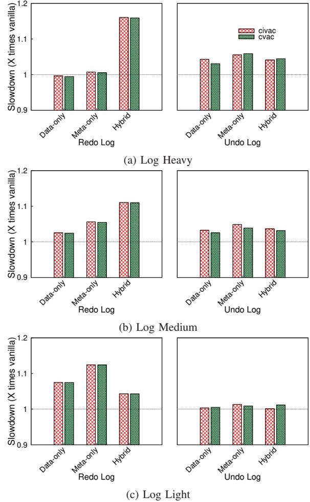
Fig. 8: Arm64: Influence of data consistency methods based on nature of update operations for different logging requirements. Y-axis values are slowdown w.r.t. vanilla case of no logging (lower the better).
