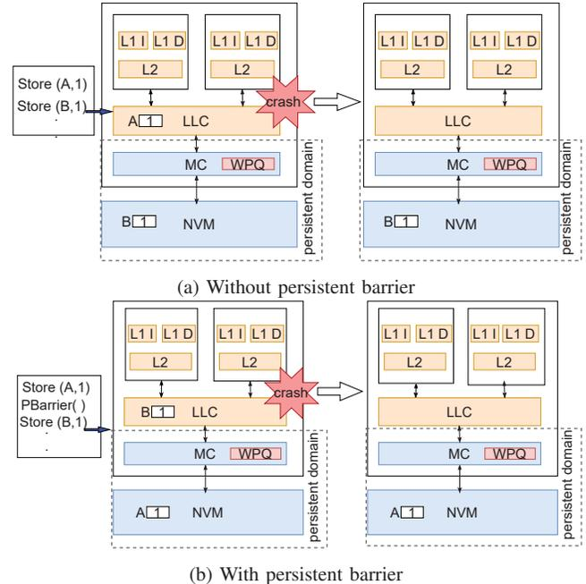
Fig. 1: Consistency issue with non-volatile memory and solution using persistent barrier (shown as PBarrier) techniques. [A, B - NVM Addresses, Store(A, 1) - writes 1 to NVM address A]
