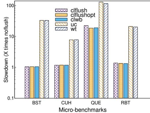
Fig. 4: Performance overhead of data consistency methods. Y-axis values are slowdown with respect to not using any data consistency method (lower the better).
