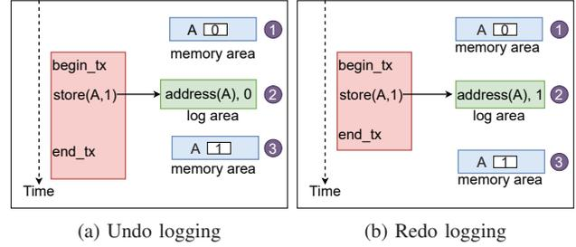
Fig. 3: Working example of undo and redo logging approaches for NVM consistency. (1) shows initial value of A, (2) shows logged information [Address of A, value], and (3) shows modified value of A.
