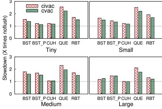
Fig. 6: Performance slowdown with different data consistency methods in Arm64 systems. Y-axis values are slowdown normalized to noflush (lower the better)
