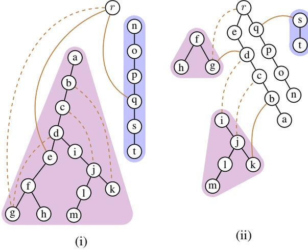
Figure 4: Visiting a super vertex from  $\mathcal{T} \cup \mathcal{P}$ . (i) The algorithm visits  $T(a) \in \mathcal{T}$  using the edge  $(r, e)$  and the  $path(n, t) \in \mathcal{P}$  using the edge  $(r, q)$ . (ii) Traversal extracts  $path(e, a)$  and  $path(q, n)$  and augments it to  $T^*$ . The unvisited segments are added back to  $\mathcal{T}$  and  $\mathcal{P}$ .
