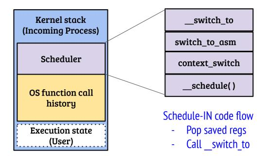
\_\_switch\_to performs bulk of state switching (including the change of per-CPU current process value)
