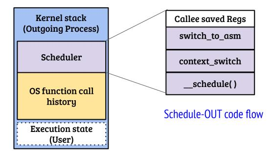
The kernel stack switch occurs in switch\_to\_asm after saving the registers into the outgoing process kernel stack
