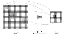
Figure 2: Back propagating deltas. A connection between two maps from two consecutive layers is displayed. The map in  $L^{n-1}$  has 29 x 29 neurons; the map in  $L^n$  has 13 x 13 neurons. They are linked through a 5 x 5 kernel K. Skipping factors of  $S_x = 1$  and  $S_y = 1$  are assumed. Arrows and colors depict the correspondence between neurons in  $L^{n-1}$ and their sources in  $L^n$ .
