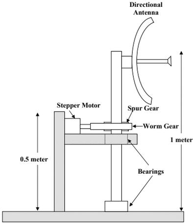
Figure 3.10: Mounting prototype
