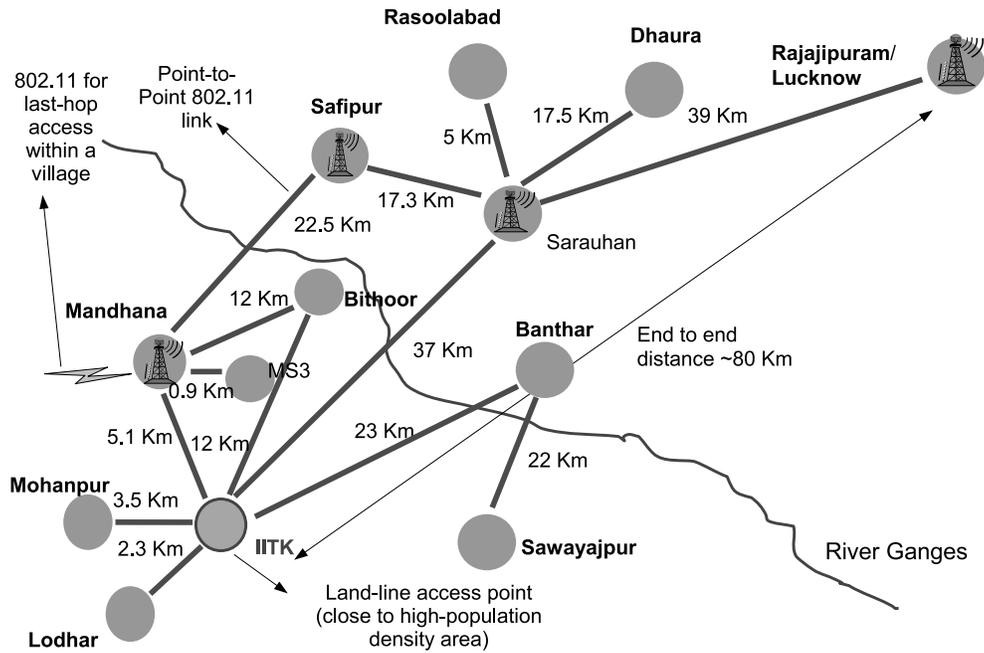
Figure 1.1: Digital Gangetic Plains Testbed
