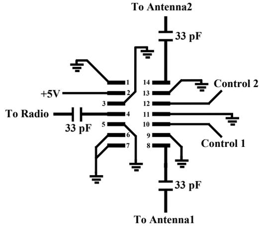
Figure 3.4: RF-Switch with RSW-2-25-P
