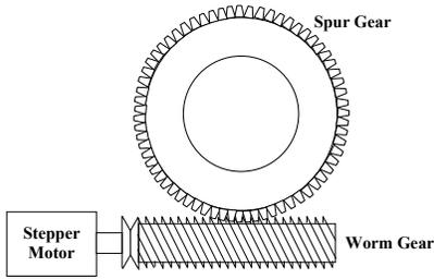
Figure 3.11: Spur Gear and Worm Gear
