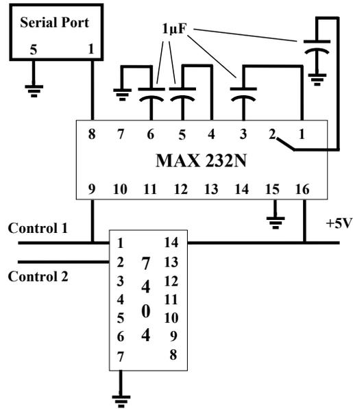
Figure 3.5: Hardware for generating control logic
