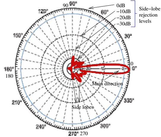
Figure 3: Spatial radiation pattern of parabolic grid antennae
