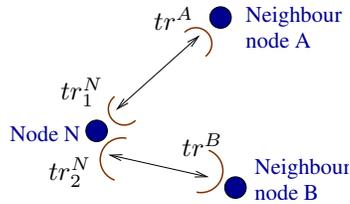
Figure 2: Multiple directional antennae at a node
