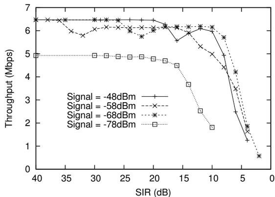
Figure 5: Throughput variation with decreasing interference
