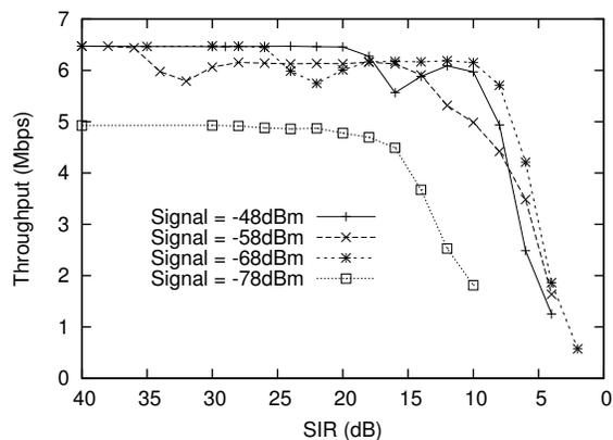
Figure 5: Throughput variation with decreasing interference
