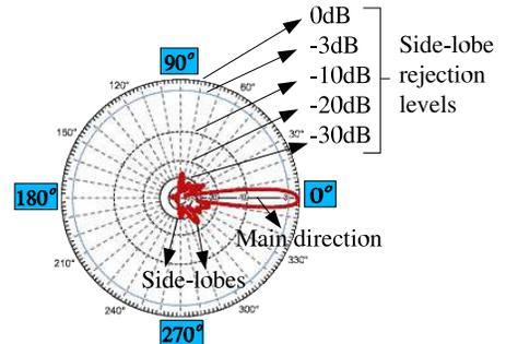
Figure 10: Spatial radn. pattern: parabolic grid antenna
