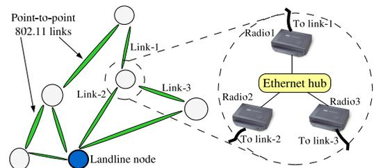
Figure 1: 802.11 mesh: nodes have one radio per link
