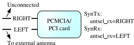
Figure 5: Using *antsel\_rx* to avoid carrier-sensing
