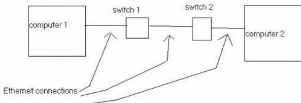
Then it is not possible to detect a failure if the link between switch1 and computer1 fails.
