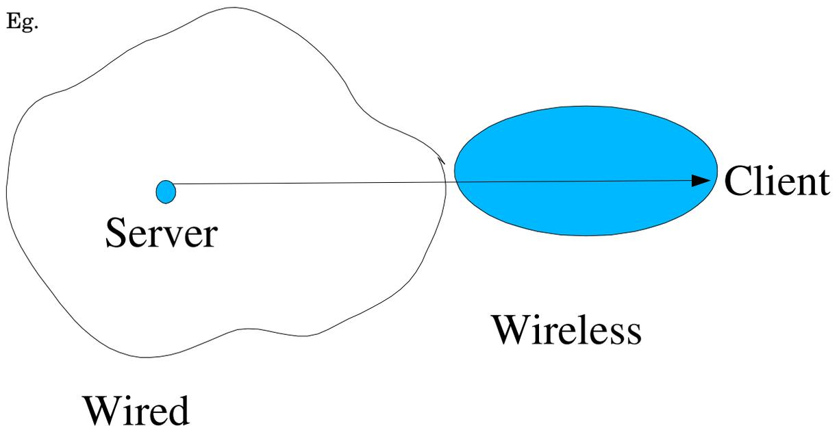
TCP doesn't perform well on wireless networks as it was designed basically for wired networks. To improve performance a large number of optimizations have been done in the network layer.
