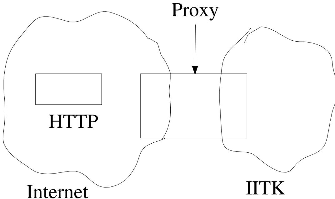
Diagram shows that a Proxy Server has been introduced between Internet and IITk network.
