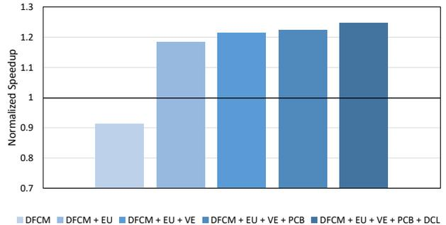
Figure 3: Normalized speedup with the enhancements on DFCM (early update, value estimator, PC blacklister, dynamic context length). Note that additional 4% gain is achieved by fine tuning the enhancements and the associated policies.
