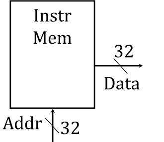
Reads are combinational: Put a stable address on input, a short time later data appears on output.
