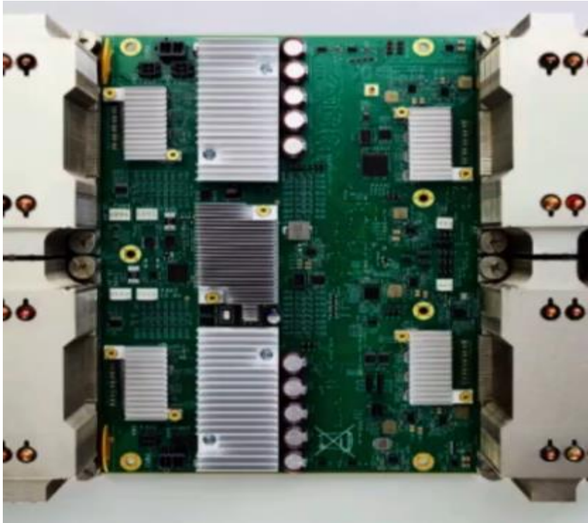
Figure 3. TPU Printed Circuit Board. It can be inserted in the slot for an SATA disk in a server, but the card uses PCIe Gen3 x16.
