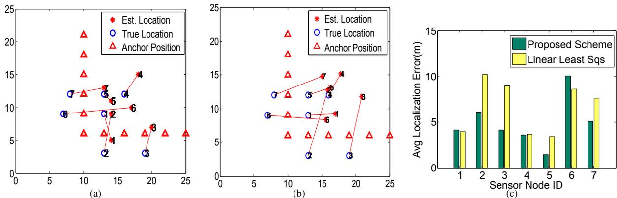
Fig. 6. (a) Experiment scenario where triangles are the positions of the anchors using our proposed scheme. (b) Using Linear Least Square Method. (c) Comparison of average localization error for each node of these two schemes.
