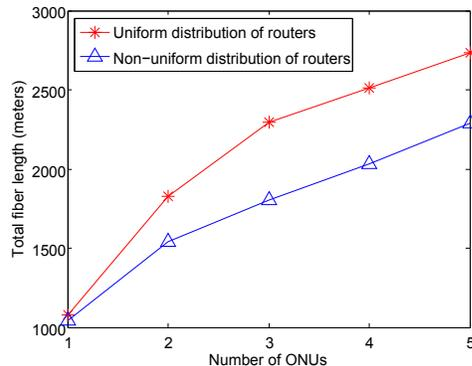
Fig. 15. Comparison of total fiber length required for tree PON architecture for uniform and non-uniform distribution of mesh routers.
