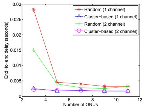
Fig. 12. Comparison of end-to-end delay with different number of ONUs for random placement and clustering-based schemes for non-uniform distribution of mesh routers.
