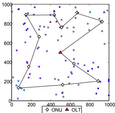
Fig. 16. Fiber layout by solving the travelling salesman problem for uniform distribution of mesh routers.
