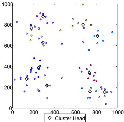
Fig. 8. The placement of eleven ONU with cluster-heads where mesh routers are non-uniformly distributed.
