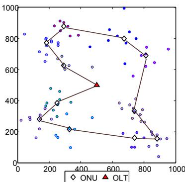
Fig. 17. Fiber layout by solving the travelling salesman problem for non-uniform distribution of mesh routers.
