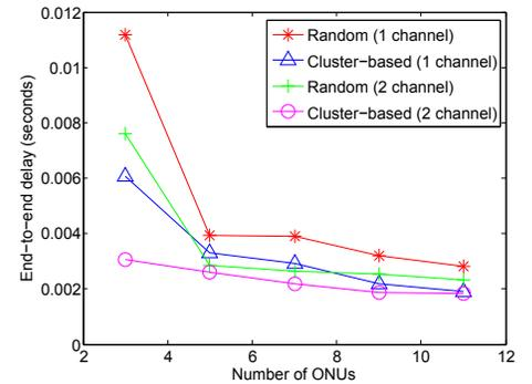
Fig. 7. Comparison of end-to-end delay with different number of ONUs for random placement and clustering-based schemes for uniform distribution of mesh routers.
