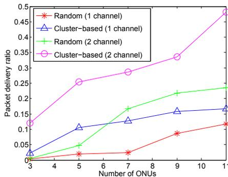
Fig. 11. Comparison of delivery ratio with different number of ONUs for random placement and clustering-based schemes for non-uniform distribution of mesh routers.
