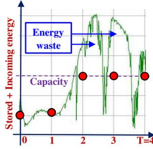
Fig. 3. Energy wastage due to lack of storage capacity. Red dots are the actual energy.
