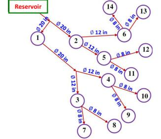
Fig. 4. Simulation topology, red arrows show the direction of water-flow [3].
