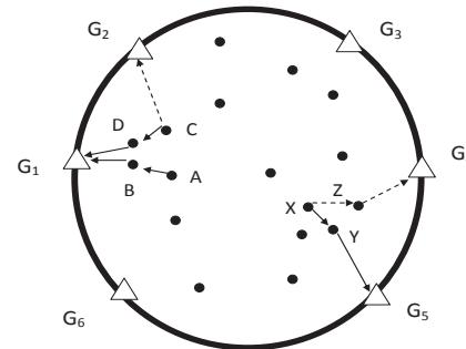
Fig. 1. Wireless mesh network architecture with multiple gateways
