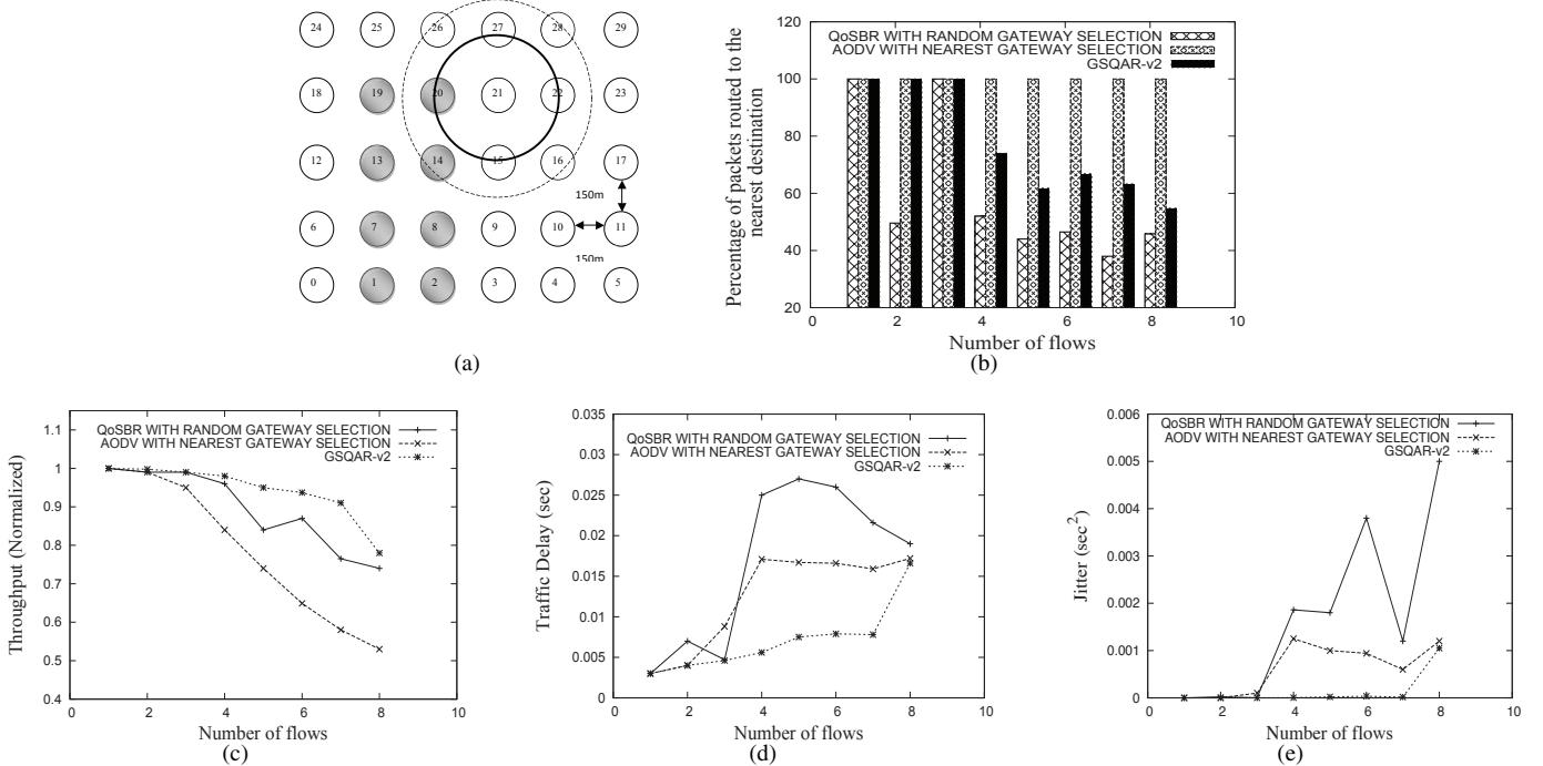
Fig. 5. (a) Simulation scenario, 19, 20, 13, 14, 7, 8, 1, 2 are activated in sequence, 24 and 29 are gateways, interference and transmission range are dotted and dark circle respectively (b) Comparison of percentage of packets routed to the nearest gateway (c) Throughput (d) Delay (e) Jitter.
