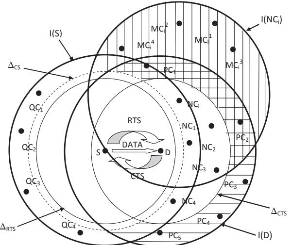
Fig. 2. Effect of interferers in presence of RTS/CTS for test link  $S \rightarrow D$
