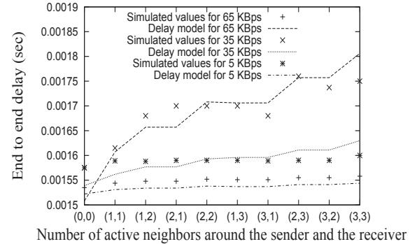
Fig. 3. Variation of delay with different number of active neighbors of sender and receiver. The terms in x axis are  $(n_a, n_b)$ .
