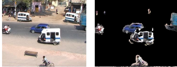
Figure 2.2: Segmentation is free, but noisy. A frame from a traffic video, and the extracted foreground blobs. Blobs like the tempo-car occlusion are identified as occlusions during tracking. Only isolated tracks are considered for object discovery.
