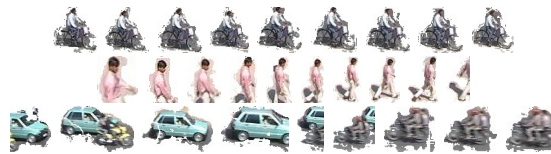
Figure 2.3: Agents as sequences of isolated foreground blobs. Bottom row (agent 130): the sequence is initially tracking a car - but after it exits, it is erroneously mapped to a motorcycle.
