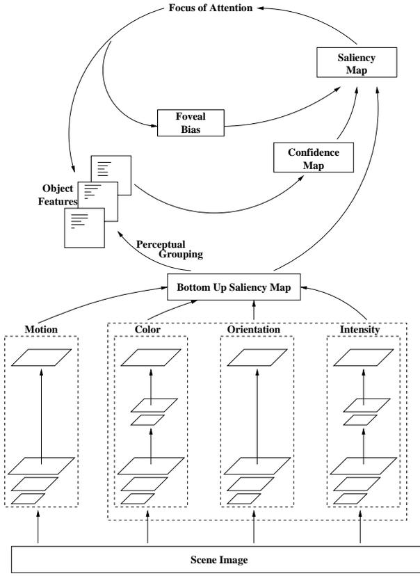
Fig. 2. *Bottom-Up Dynamic Visual Attention Model*. The feature maps for static images (colour, intensity and orientation) are extended with a motion saliency map (based on optical flow). In addition a confidence map records which sites have not been visited for a longer time. Winner-Take-All determines the next fixation.
