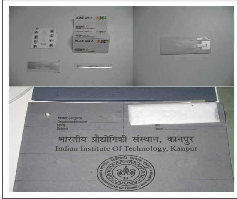
Figure 4.1: RFID Tag Packaging and Placement on the File
