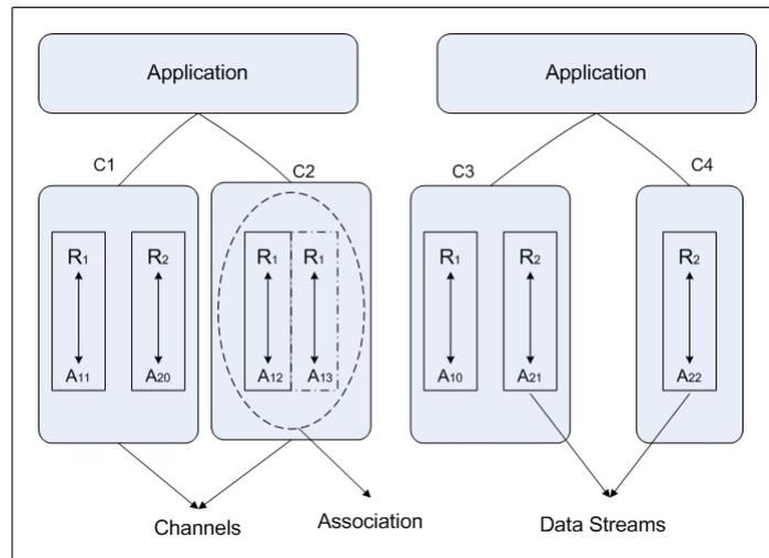
Figure 3.3: Channels- Grouping of Data Streams
