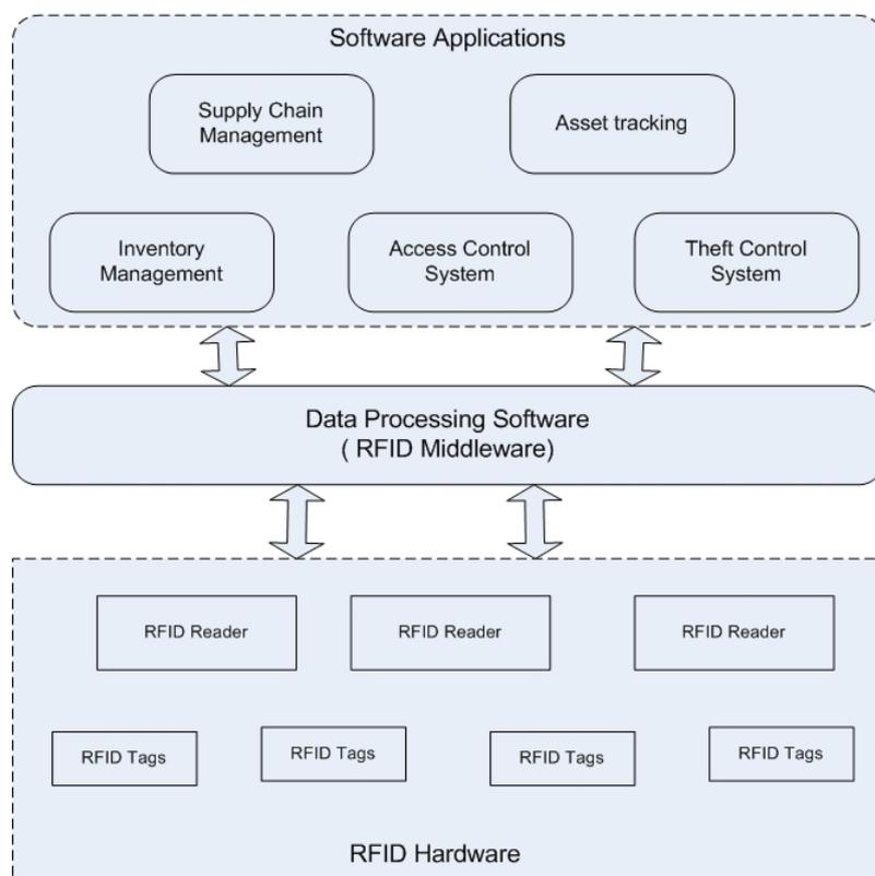
Figure 2.1: RFID System Components
