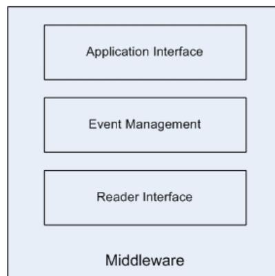
Figure 2.2: Components of RFID Middleware
