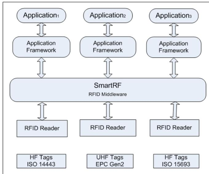
Figure 3.1: System Architecture
