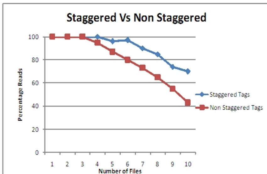
Figure 4.7: Comparison between Staggered and Non-Staggered Positioning
