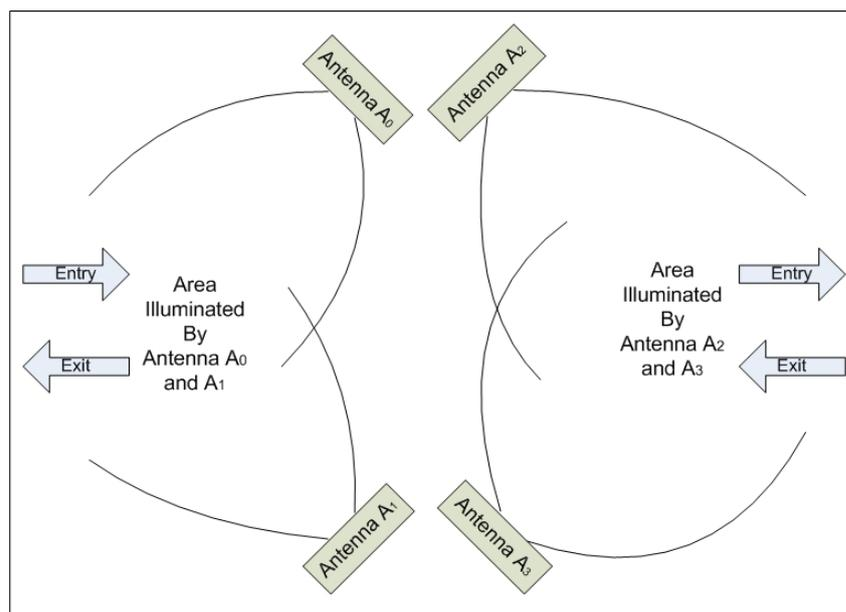
Figure 4.2: Antenna Placement and Orientation at the Room Entrance
