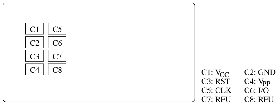
Figure 1.1: Physical interface of smart card
