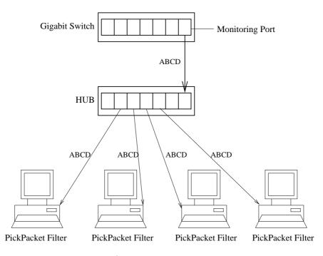
Figure 3.1: The Architecture of Hub based approach
