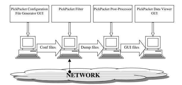
Figure 2.1: Architecture of PickPacket
