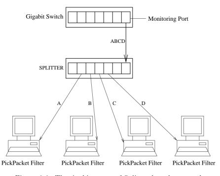
Figure 3.3: The Architecture of Splitter based approach
