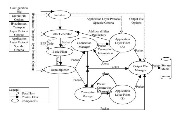
Figure 2.3: The Basic Design of the PickPacket Filter
