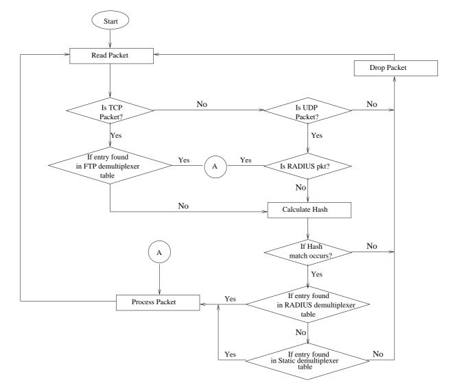
Figure 3.2: Packet handling in Hub based approach
