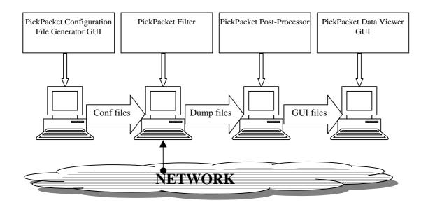
Figure 2.1: The Architecture of PickPacket [15]
