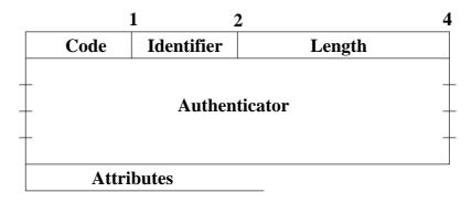
Figure 3.2: RADIUS Packet Format
