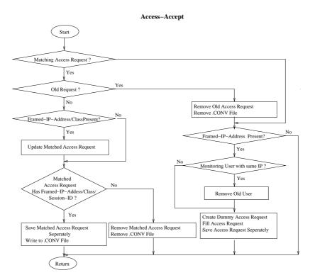
Figure 4.7: Access-Accept Packet Post-Processing
