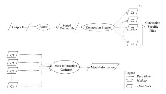
Figure 2.4: Post-Processing Design [10]
