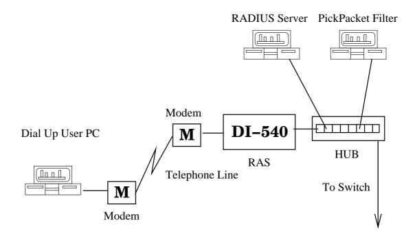
Figure 5.1: RADIUS Test Setup
