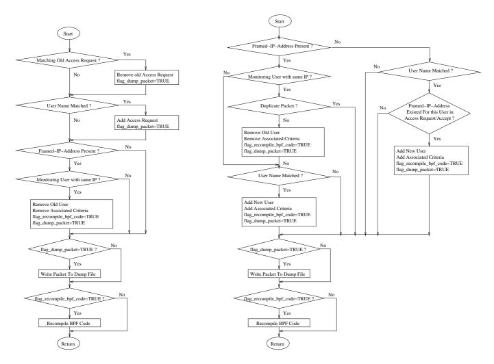
Figure 4.2: Access-Request Packet Processing by RADIUS Filter
