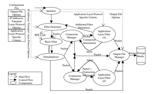
Figure 2.3: The Basic Design of the PickPacket Filter [10]
