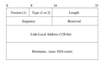
Figure 10: Format of Client Request Packet
