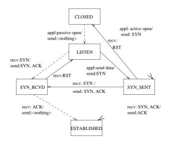
Figure 2: TCP State Processing during Initial Handshake
