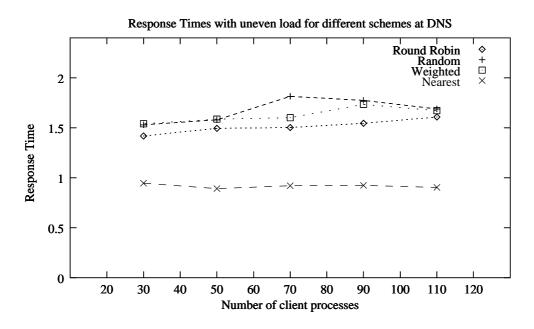
Figure 5.6: Average response time (uneven load) with different policies used at DNS
