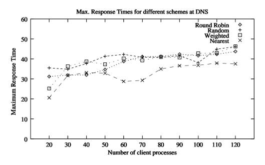
Figure 5.7: Maximum response time with different policies used at DNS
