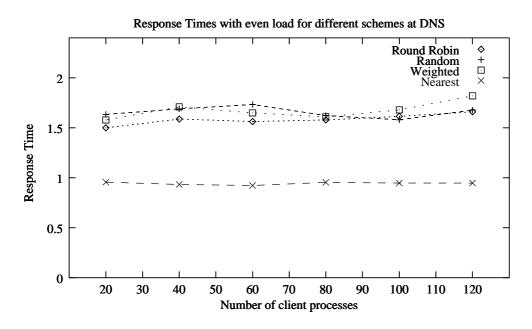
Figure 5.5: Average response time (even load) with different policies used at DNS
