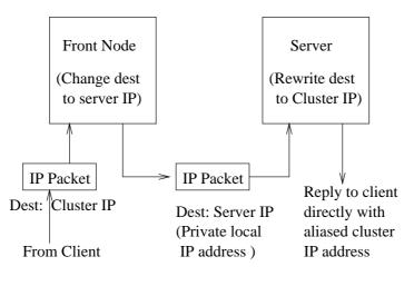
One way IP packet forwarding by Front node using divert socket at application layer
