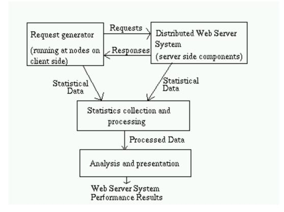
Figure 4.1: Block diagram of Test bed
