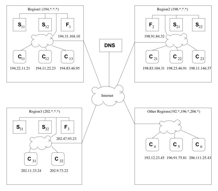
Figure 4.2: Test bed used in Experiments
