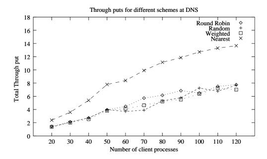
Figure 5.9: Total through put with different policies used at DNS
