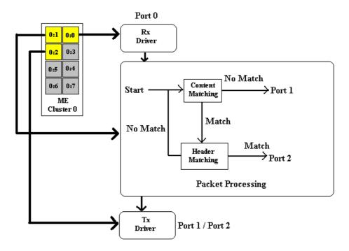
The Structure of Receive, Process and Transmit on IXP2400
