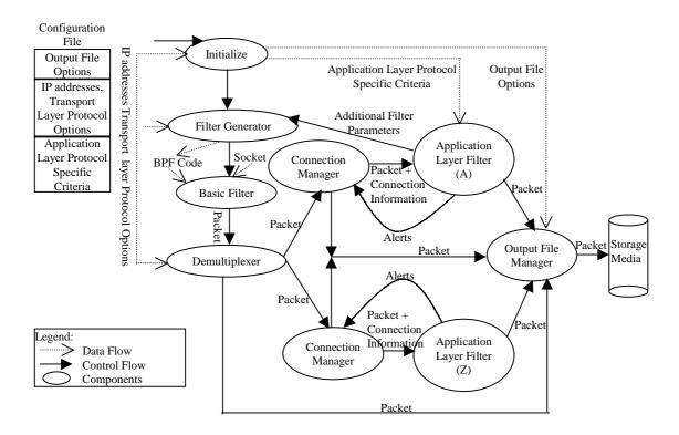
Figure 3.5: The Basic Design of the PickPacket Filter
