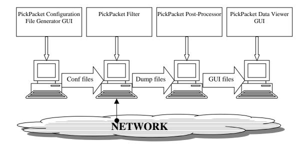
Figure 3.1: The Architecture of PickPacket
