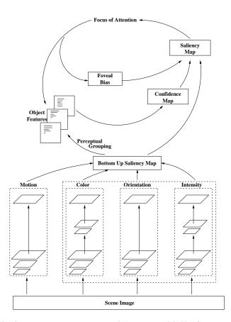
Fig. 2. Bottom-Up Dynamic Visual Attention Model. The feature maps for static images (colour, intensity and orientation) are extended with a motion saliency map (based on optical flow). In addition a confidence map records which sites have not been visited for a longer time. Winner-Take-All determines the next fixation.
