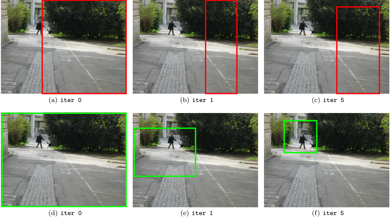
Fig. 9 Cropping operation on a ‘person’ labeled image for various iterations during training. The first and second rows show the result of the ordinary and iterative learning respectively. The first learning algorithm misses the ‘person’ in the first iteration and later converges to some part of background. The same local minimum is avoided in the second learning algorithm by restricting the possible image windows set to the full image in the first iteration and gradually relaxing the restriction.
