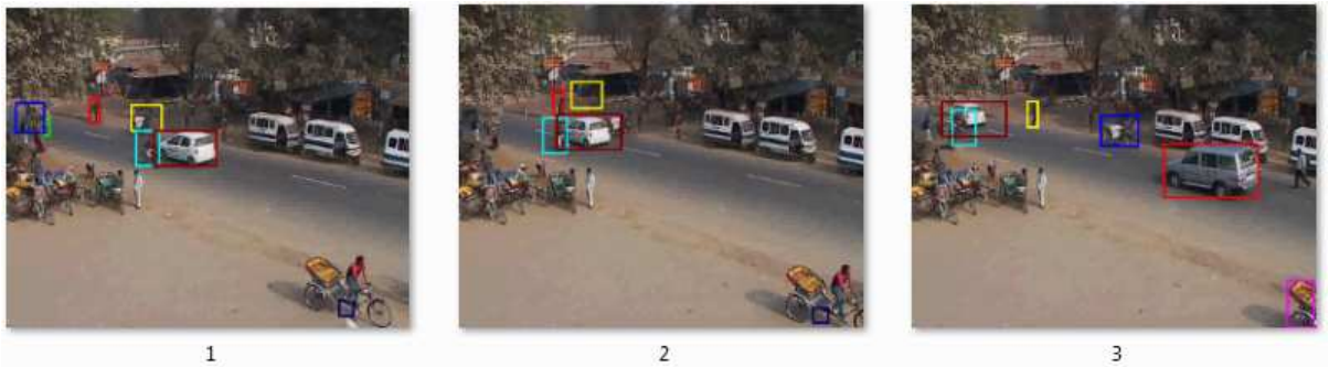
Figure 7: This is the result of mean shift tracking implemented by P. Guha in IITK. (1) shows a car marked by maroon box and a rickshaw by yellow, (2) shows that due to occlusion by car the rickshaw is not marked and the yellow box of rickshaw is not having object in it, (3) Rickshaw is identified as a new object (marked by blue box) and yellow box marks a person which earlier was marked by red box.
