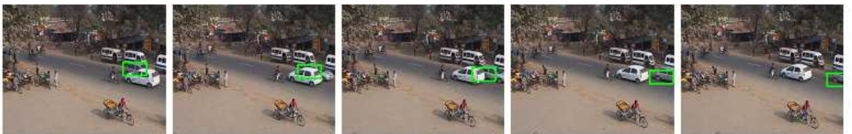
Figure 2: Dynamic Occlusion: moving grey car is occluded by another moving white car
