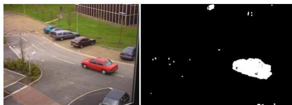
Figure 5: The original image on left and the the output after running our background subtraction code
