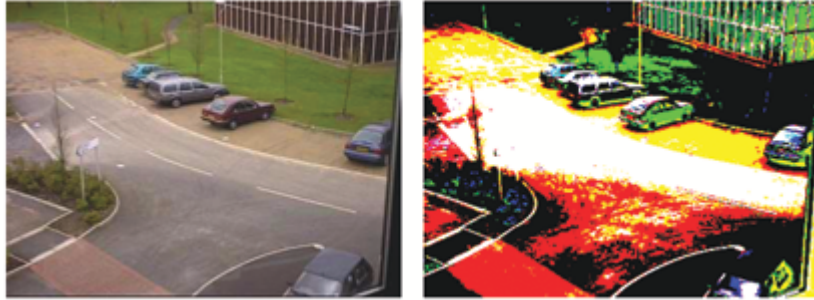
Figure 3: The likelihood image obtained by mean and variance. The threshold T is taken as 1.0. The R component value is set to be 255 in output image to the pixels with \psi_R component greater than 0 in input image, the G component value is set to be 255 in output image to the pixels with \psi_G component greater than 0 in input image and the B component value is set to be 255 in output image to the pixels with \psi_B component greater than 0 in input image.
