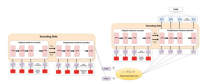
Figure 2: The block diagram of our VAE-LSTM architecture for paraphrase generation
