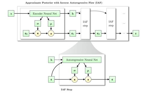
**Figure 3.1:** Like other normalizing flows, drawing samples from an approximate posterior with Inverse Autoregressive Flow (IAF) (Kingma *et al.*, 2016) starts with a distribution with tractable density, such as a Gaussian with diagonal covariance, followed by a chain of nonlinear invertible transformations of z, each with a simple Jacobian determinant. The final iterate has a flexible distribution.
