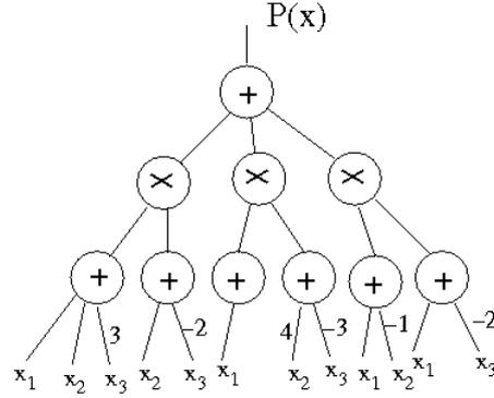
Figure 2.2: A depth-3 circuit.
