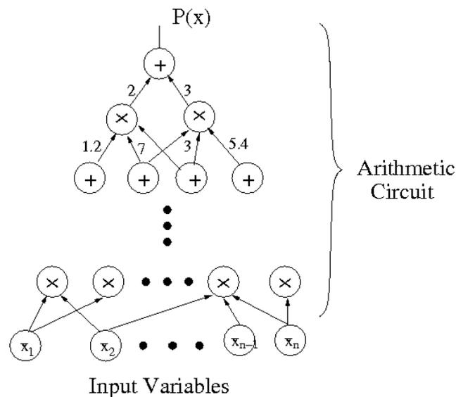
Figure 2.1: An arithmetic circuit.
