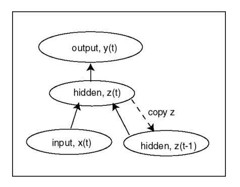
The Elman network commonly is a two-layer network with feedback from the first-layer output to the first layer input. This recurrent connection allows the Elman network to both detect and generate time-varying patterns.
