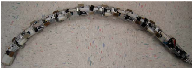
Fig. 9 Snake robot in its rolling arc configuration
