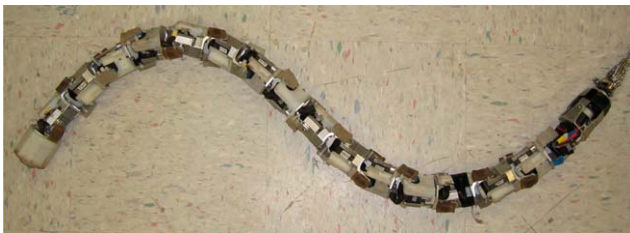
Fig. 13 Snake robot in its rolling “S” configuration
