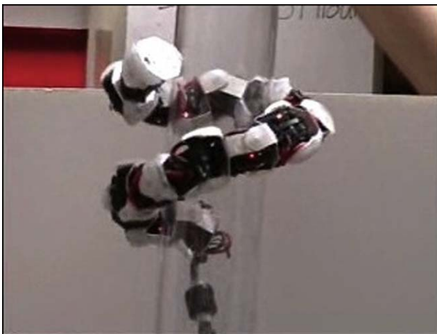
Fig. 1 Our modular snake ("modsnake") robots have sixteen joints, arranged to allow full workspace flexibility. In past work, we have demonstrated a variety of successful motion strategies for these robots, including traversal of both smooth and rough terrain, swimming, and pole climbing (shown here)
