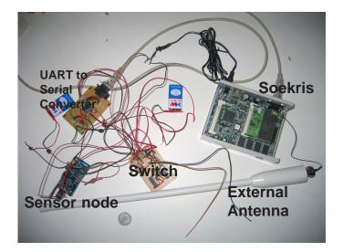
Figure 3.1: Circuit of Base Node developed by us
