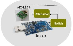
Figure 1.2: Components of a single sensor node
