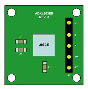
Figure 3.4: Physical layout of the ADXL203 Evaluation Board
