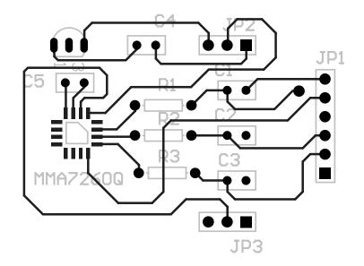
Figure 3.3: Application circuit for MMA7260Q accelerometer chip
