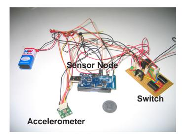
Figure 3.2: Circuit of Node developed by us
