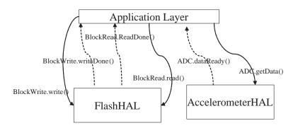
Figure 2.7: Interaction between application Flash and the Accelerometer
