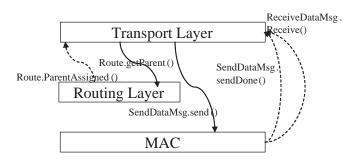
Figure 2.8: Interaction between transport layer, Routing and MAC
