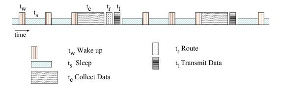
Figure 2.4: Timeline diagram of the wireless sensor network
