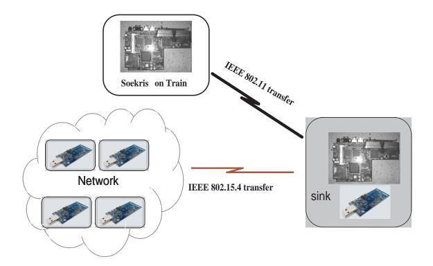
Figure 1.5: Application Design of the Entire Network
