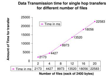
Figure 6.4: Plot of data transfer duration vs number of files
