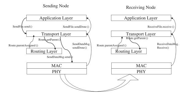
Figure 2.5: Application stack of a node sending a file from one node to another
