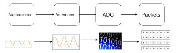
Figure 1.4: Application Design of a Single Node
