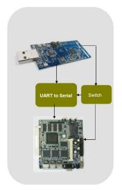
Figure 1.3: Components of the base node
