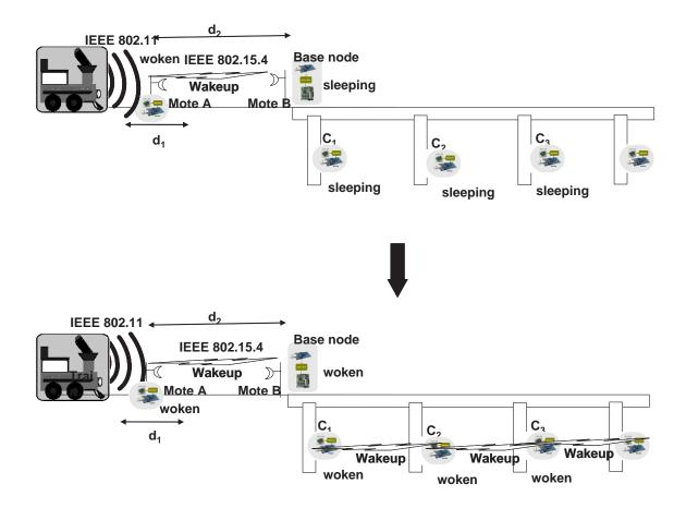
Figure 2.1: Wake up mechanism for the network
