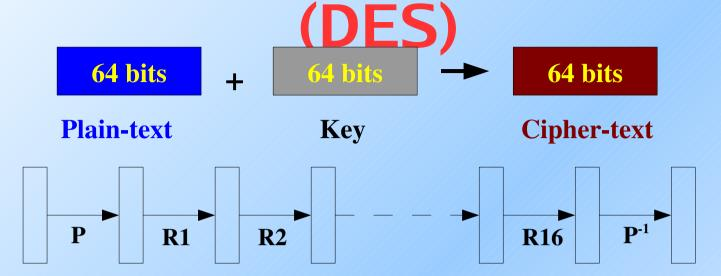
Permutation, 16 rounds of identical operation, inverse permutation
